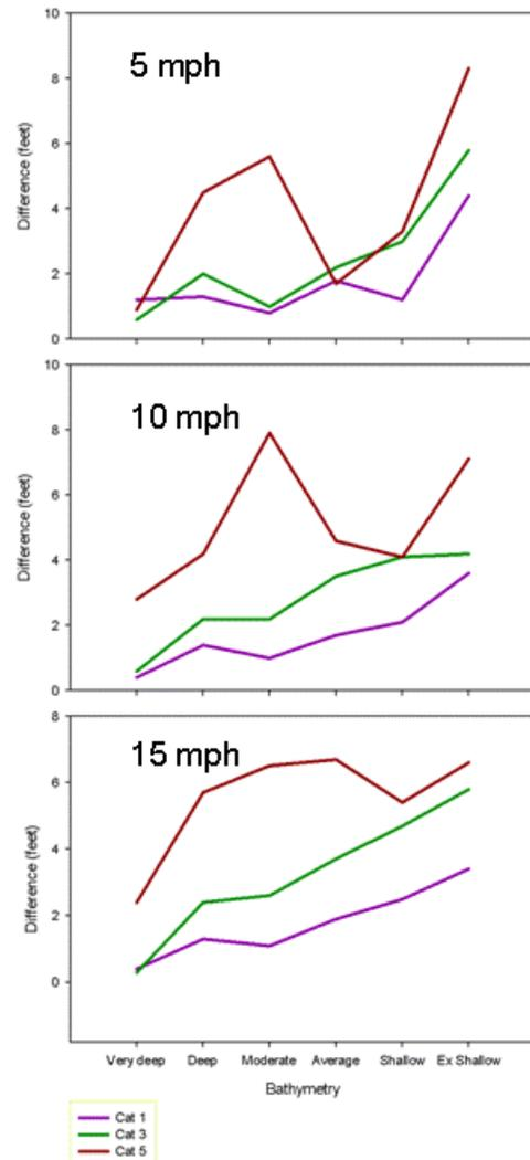
**Figure 3. (Left side) Speed influence for small, average, and large hurricanes, computed by subtracting peak surge values for fast-moving from slow-moving storms. (Right side) Size influence, computed by large minus small peak storm surges, partitioned by translation speed.**
