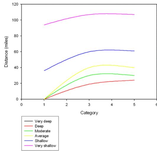
**Figure 6. Distance (miles) of 5-ft and 10-ft inundation from storm center for average-speed, average-size hurricanes as a function of intensity and bathymetry classes.**
