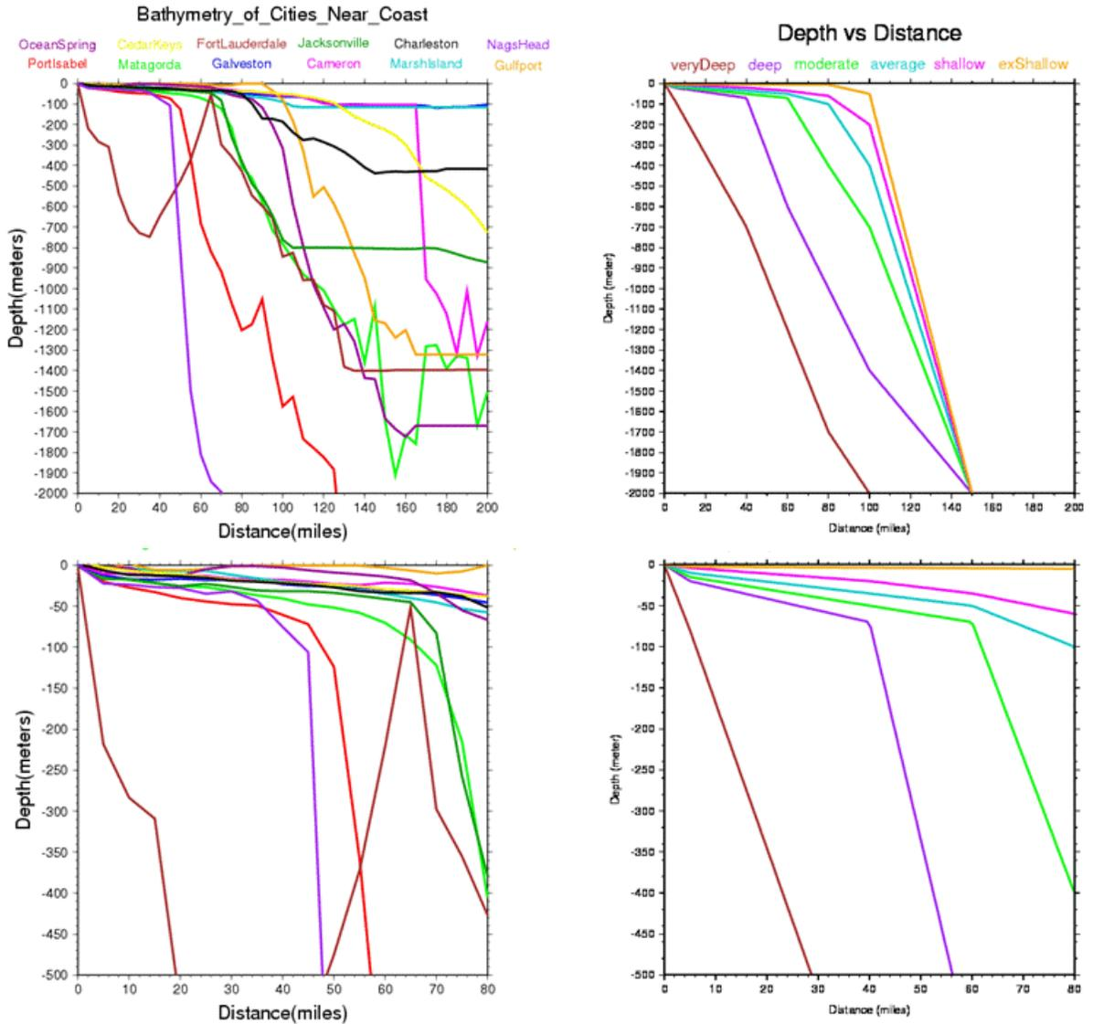
**Figure 1. Bathymetry cross-sections for 10 coastal cities out to 200 miles (top left) and zoomed in to 80 miles (bottom left) that represent a spectrum of continental slopes. Six hypothetical bathymetries based on these cities are shown ranging from close deep water to a shallow continental slope for 200 miles (top right) and 80 miles (bottom right), defined as Very Deep, Deep, Moderate, Average, Shallow, and Extremely Shallow slopes.**
